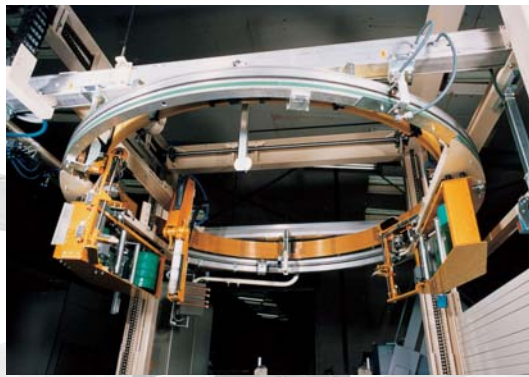
Slip ring with conductor rail system in a stretch-foil packing machine
