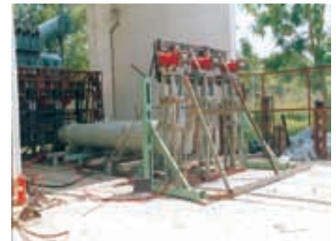
Temperature rise Testing at EDF, France
