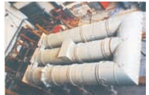
Temperature rise Testing at EDF, France
