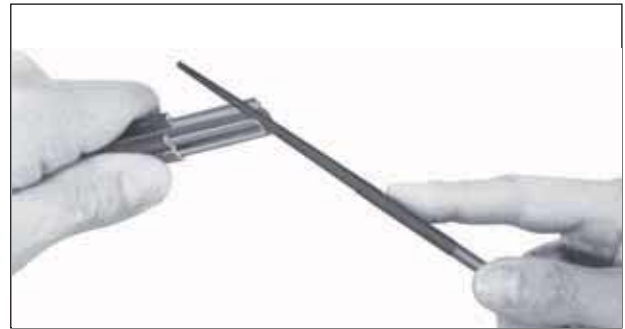
Photo 9: Remove inside burr with round file
