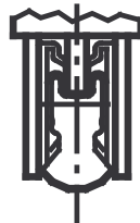
Installation Tool with position of connector Order No. 241046085
